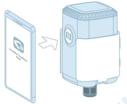
3. Click "Write" to change the configuration of EM500 and attach the smartphone with NFC area to the device until the APP shows a successful prompt.
