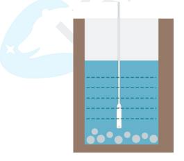
If the sensor is to be used in a well or other locations with turbulence or other disturbances, it is advisable to install a pipe to protect the sensor. Several holes should be drilled at different heights of the pipe in order to let water flow into and remove dydrodynamic pressure. **Note:** The pipe can't be placed bend.
