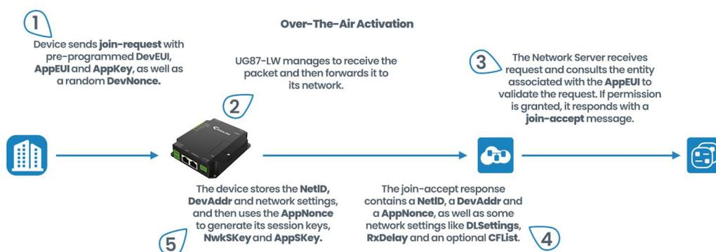
OTAA stands for Over The Air Activation. With this method the end-device sends a Join request to the gateway using the Application Key, Application Key is a shared secret key unique to your device to generate the session keys that prove its identity to the network. If the keys are correct, the gateway will reply to the end-device with a join accept message, and from that point on the
